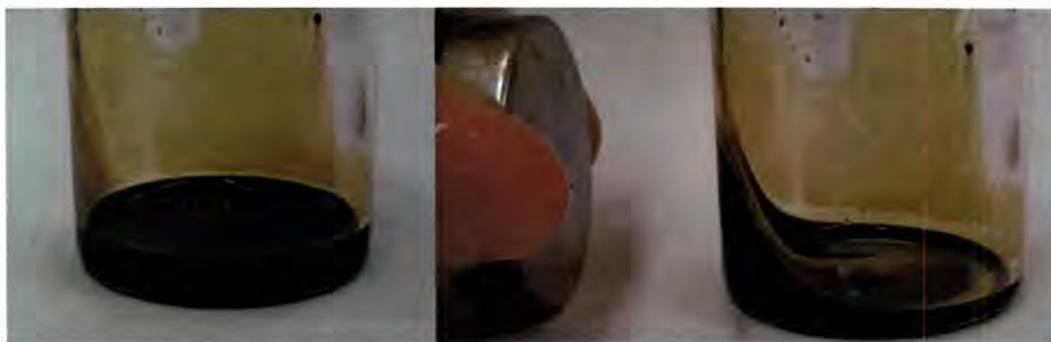
Figure 1.1. Dispersity and magnetic response of CoFe_2O_4 -RA sample after 6 months
