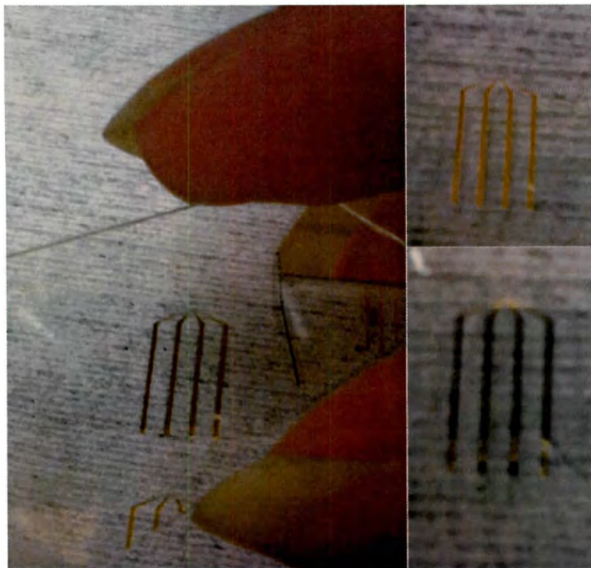
Figure 2.10. Picture of final product. Au wires deposited on fused silica with dimensions illustrated in Figure 2.5.
