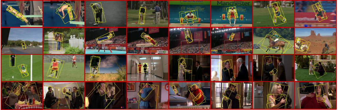
Figure 3.7: Extracted segments for example video frames from the UCF Sports and HighFive dataset. Each example frame is from a different video. The yellow boxes outlines the extracted segments. The inclusion of one box in another indicates the parent-children relationships
