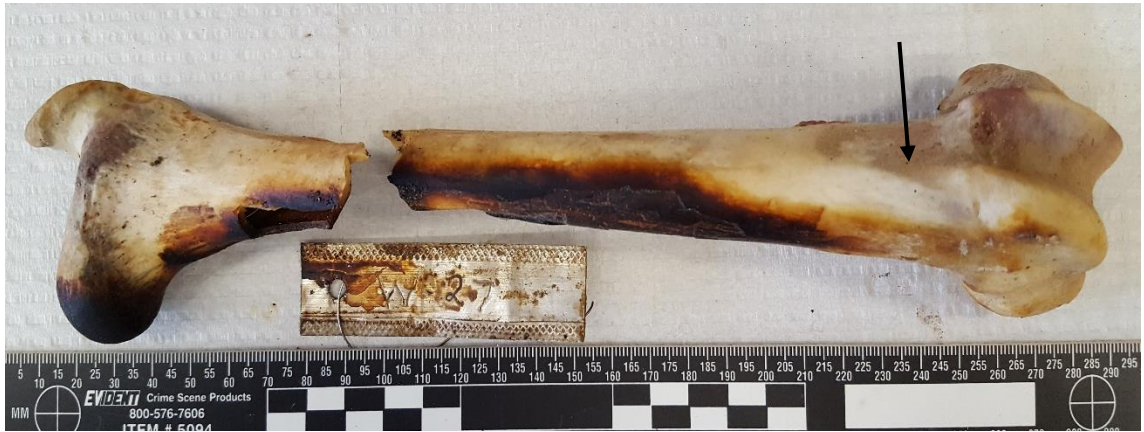
Figure 4.14. Very wet bone 27, burned elk femur with white heat line (arrow) (maximum width of 12 mm). Scale is in mm.
