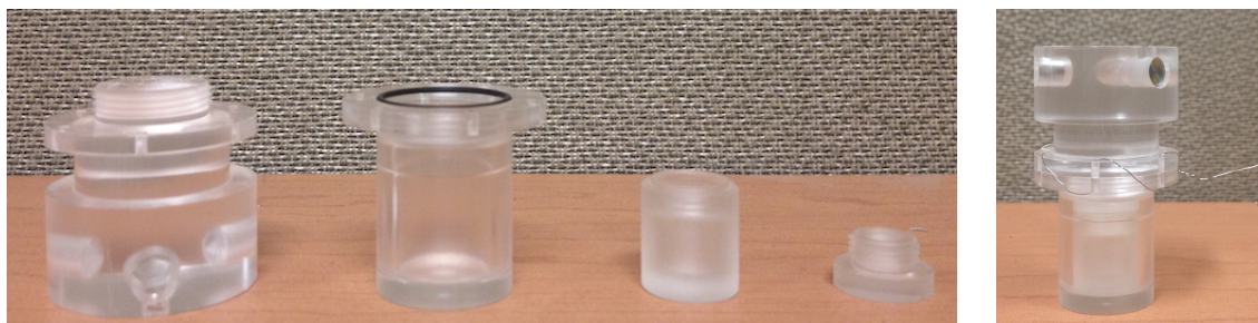
Figure 23. Left: Photo of the ^{48}\text{Sc} source components. From left to right: the lid of the outer container, the outer container with the FFKM O-ring, the inner container, and the lid of the inner container. Right: Photo of the ^{48}\text{Sc} source once closed. The safety stainless-steel wire prevents the outer container from opening while the source is moved around the detector volume. The stainless steel cross dowels are also shown (top lid).
