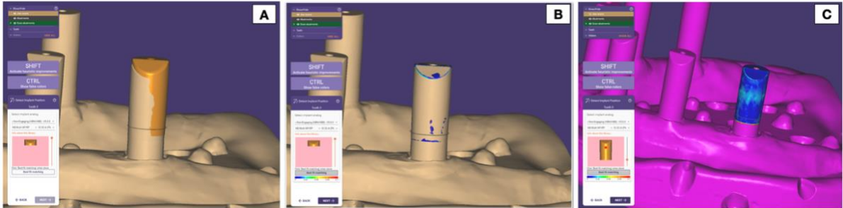
Figure 23. Scan body merged from virtual library with scanned STL using a CAD software (Exocad).
