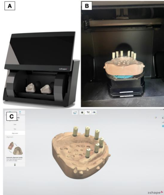
Figure 13. Scan workflow using 3ShapeD1000 (3Shape Trios) Laboratory Scanner A: 3ShapeD1000 Machine; B: Model with Scan bodies being scanned; C: Acquisition of STL file on 3Shape software.
