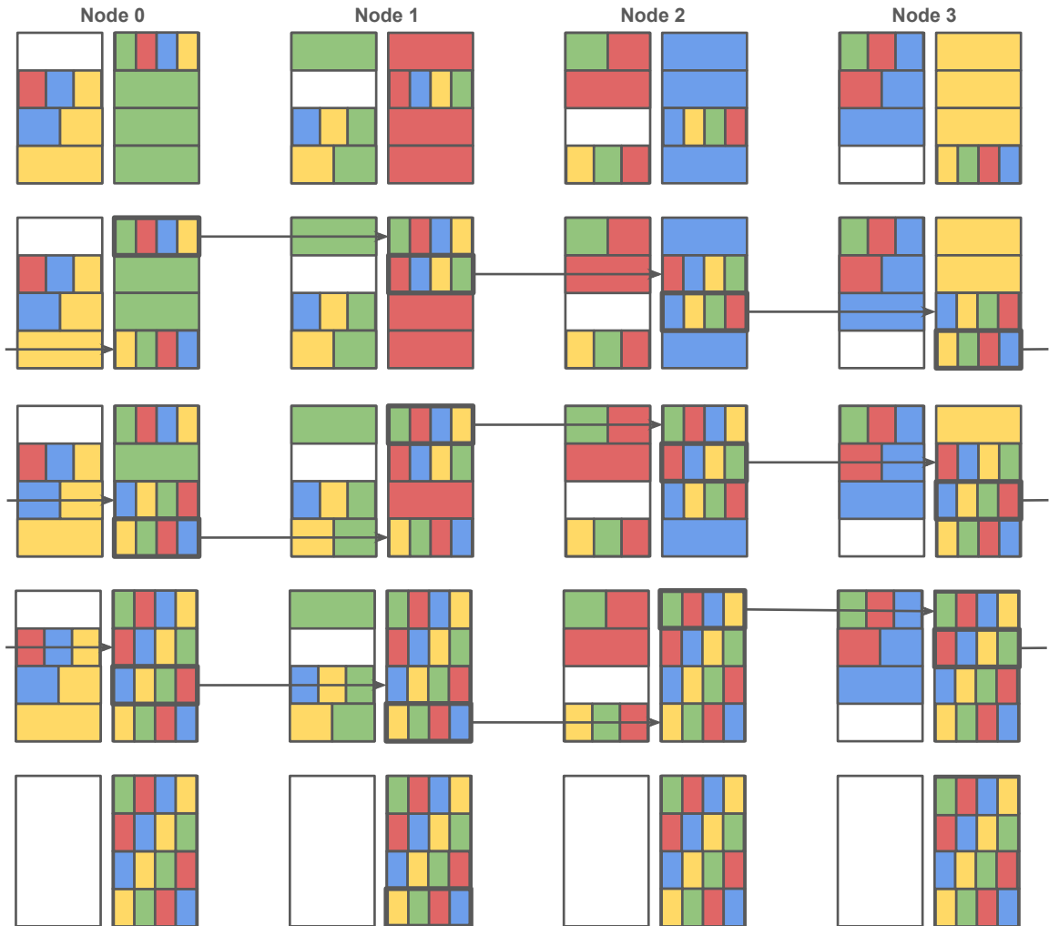
Figure 7-5: Ring-Based NCCL All-Gather Workflow.
