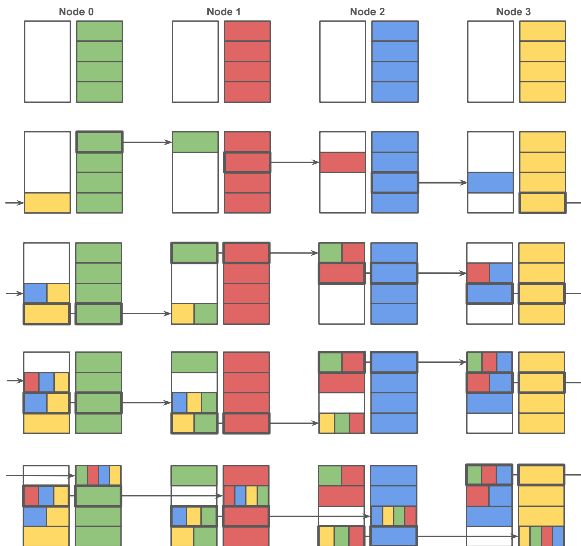
Figure 7.4: Ring-Based NCCL Reduce-Scatter Workflow.
