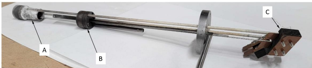
Figure 5.11: Fully assembled ball drop mechanism with coil assembly A) Coil Assembly B) Ball Loading and dropping mechanism C) Lead Attachment to connect to Arduino circuit.
