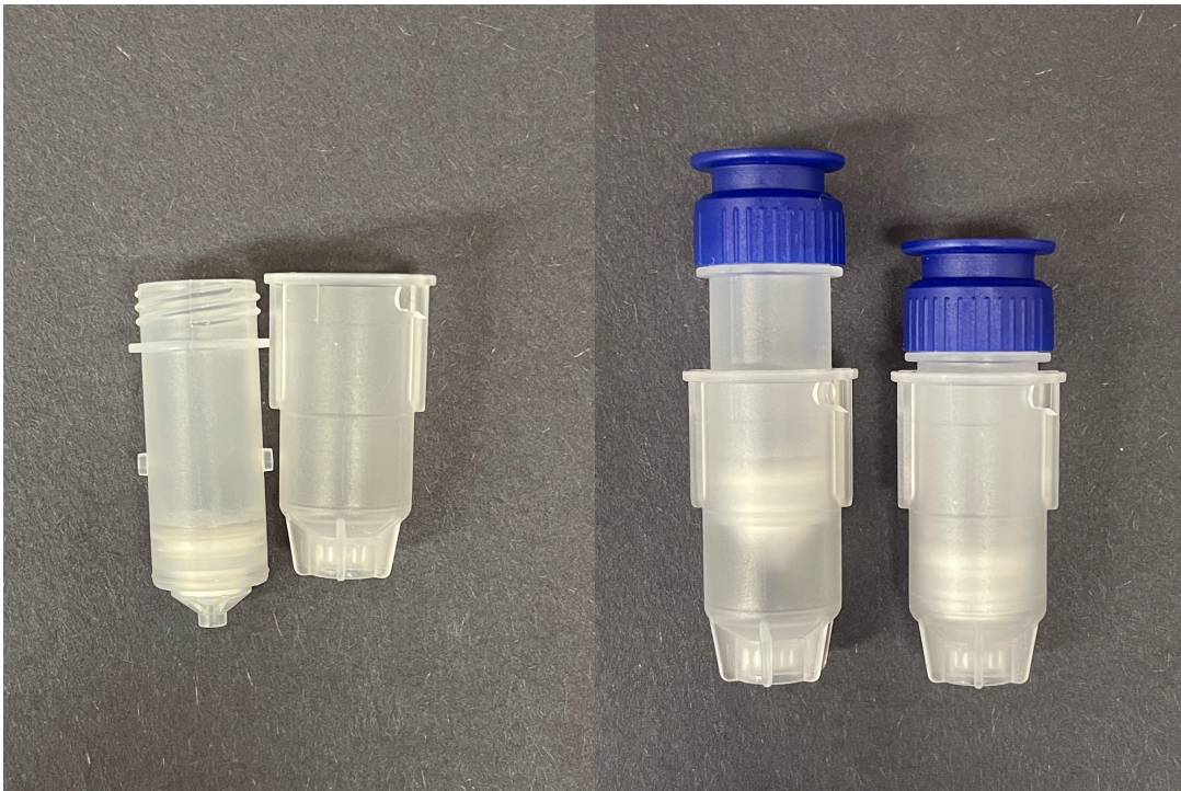
Figure 1: Depiction of SpermX™ Device in Upper and Lower Positions: Example of inner and outer tubes (left) and the assembled device (right) laid flat and in upper and lower positions.
