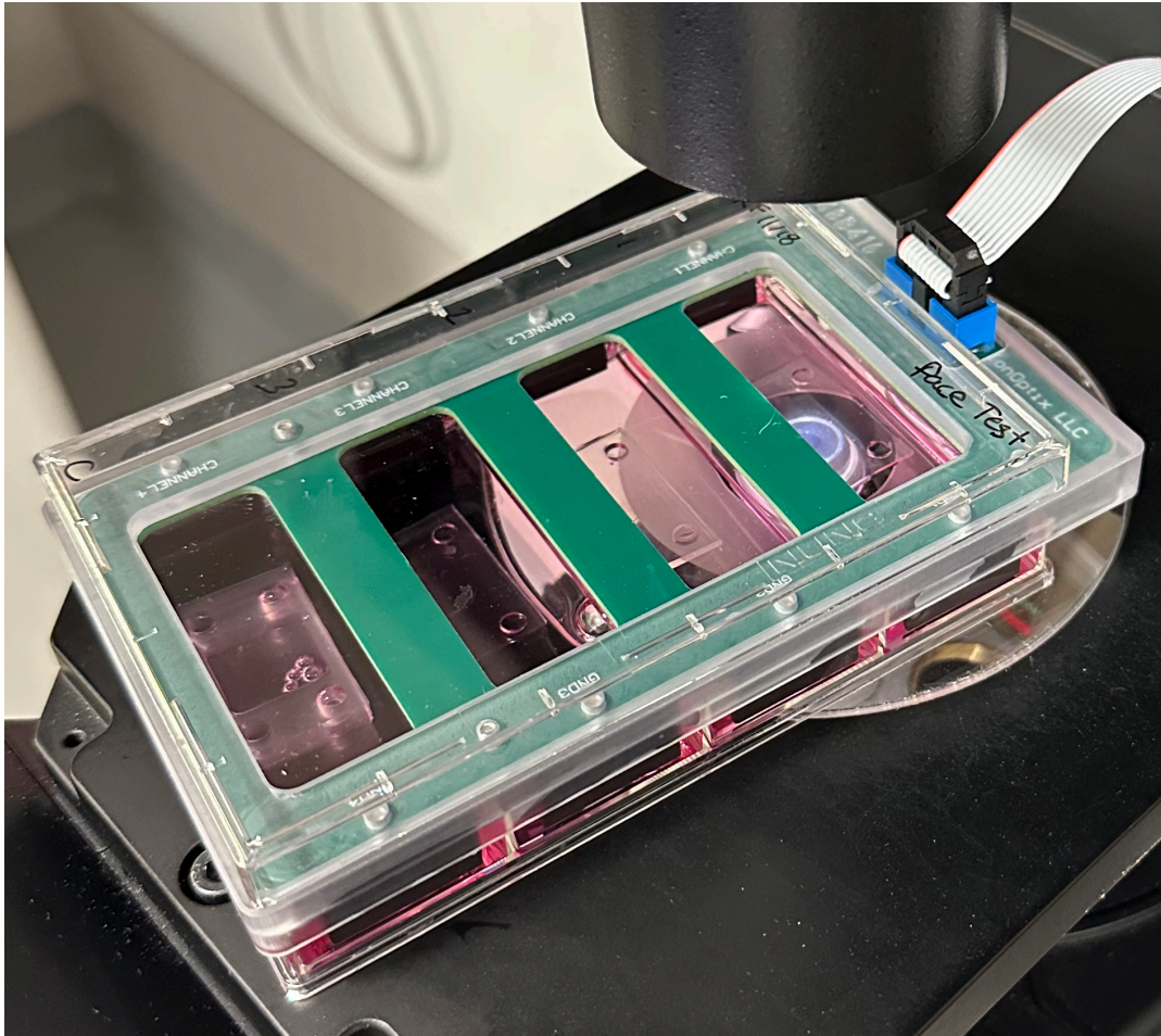
Figure 6 | Electrical pace test. The top four wells contain paced stretch layers with their stretch devices removed after fabrication, while the bottom well contains a still assembled stretch layer-device assembly as an unpaced negative control. Pacing was achieved in the three experimental layers at a 1.5 Hz frequency, 20 V amplitude, and 6 ms pulse duration.
