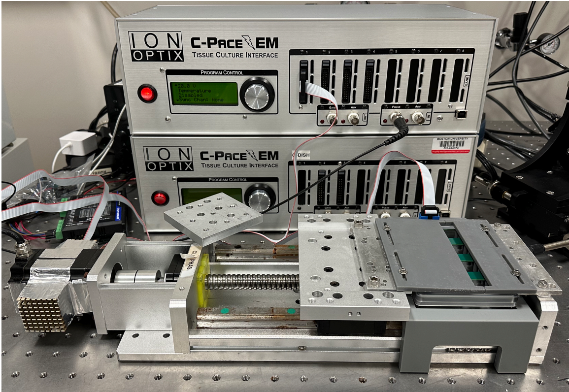
Figure 1 | Fully assembled CES platform. Complete assembly of the final Cardiomyocyte Electromechanical Stimulation Platform (CESP) ready to run experiments. The platform is capable of running integrated, synchronized electrical pacing and mechanical stretching programs to recapitulate cardiac stimuli in vitro .
