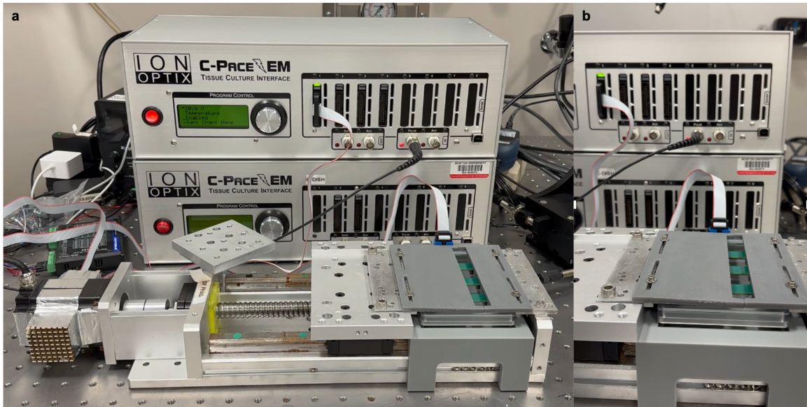
Figure 9 | Pathological delay (out-of-phase) program. The green and red indicator lights are illuminated when the stretch adapters are touching, indicating pacing during the rest phase at 0% hiPSC-cardiomyocyte monolayer strain. a , Front view. b , Side view.
