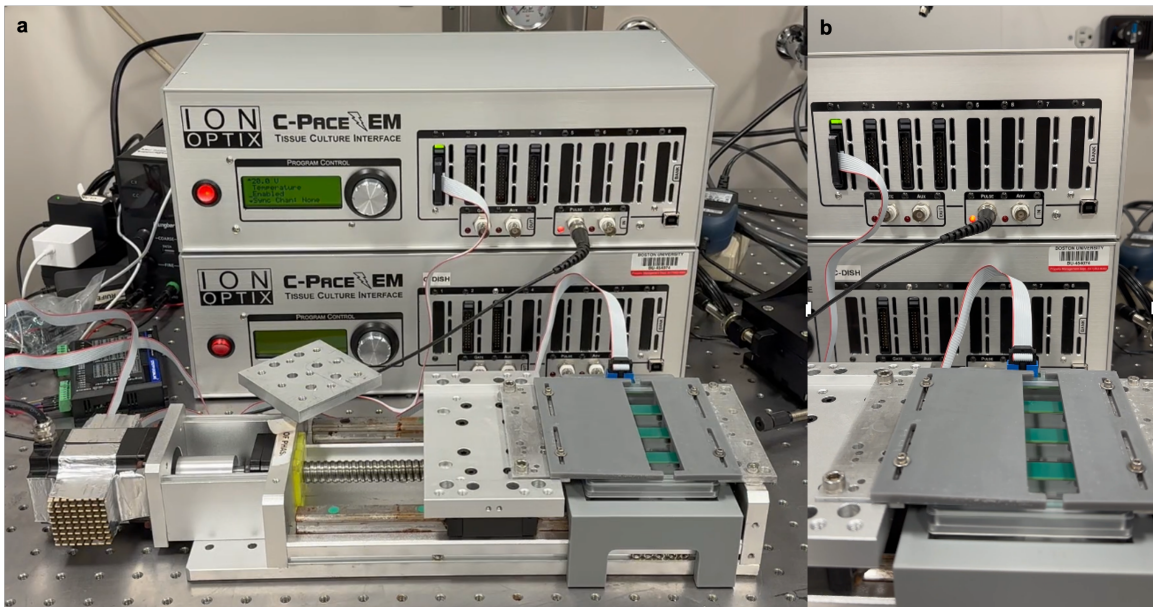
Figure 8 | Physiological delay (in-phase) program. The green and red indicator lights are illuminated when the stretch adapters are maximally separated, indicating pacing at maximum (30%) hiPSC-cardiomyocyte monolayer strain. a , Front view. b , Side view.
