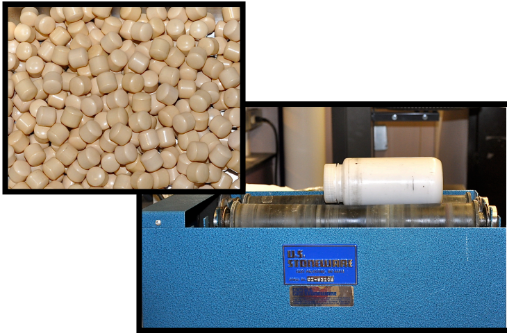
Figure 5-2: BIE powder with zirconia beads in a slow rotating milling machine for 48 hours.
