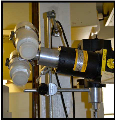
Figure 5-1: Powder mixing using a slow rotating electric motor for 24 hours.
