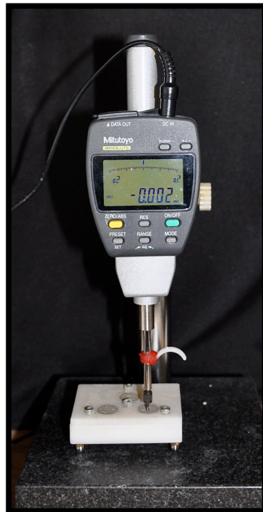
Figure 5-4: Dial indicator set up used for the setting time test.
