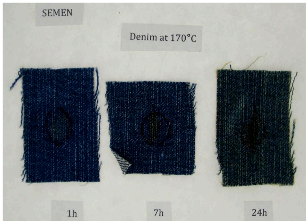
Figure 4: Semen stain on denim swatches (D2) exposed to 170°C for 1,7 and 24 hours
