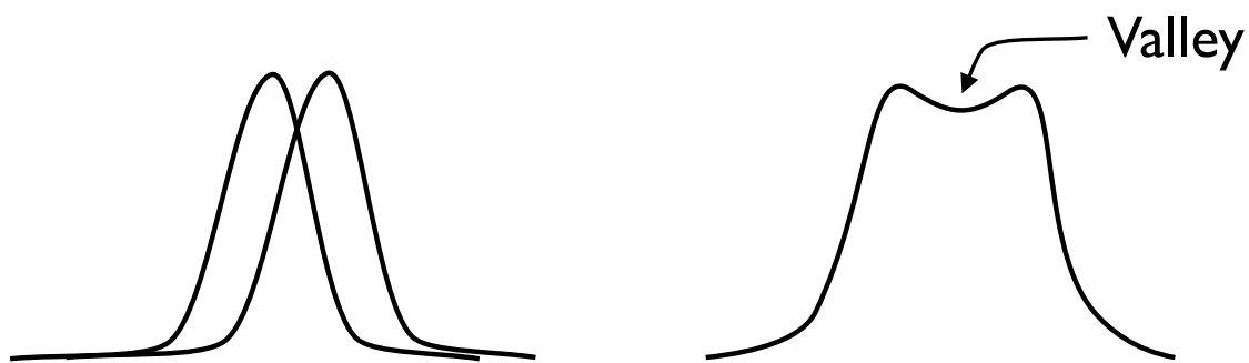
Figure 1-2: The contrast “valley” formed by the point spread functions of two nearby dots. Deciding whether the stimulus consists of one or two dots is simply a matter of being able to see the dip in contrast between the two dots.
