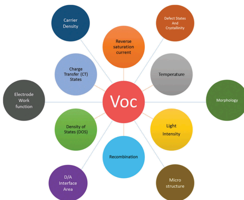
Figure 20. Parameters impacting open circuit voltage ( V_{oc} ) in OSCs (Adapted from ref. 89).
