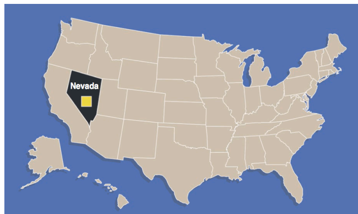
Figure 1. Area covered with 15% efficient solar cells can supply a years' worth of electricity to the United States.
