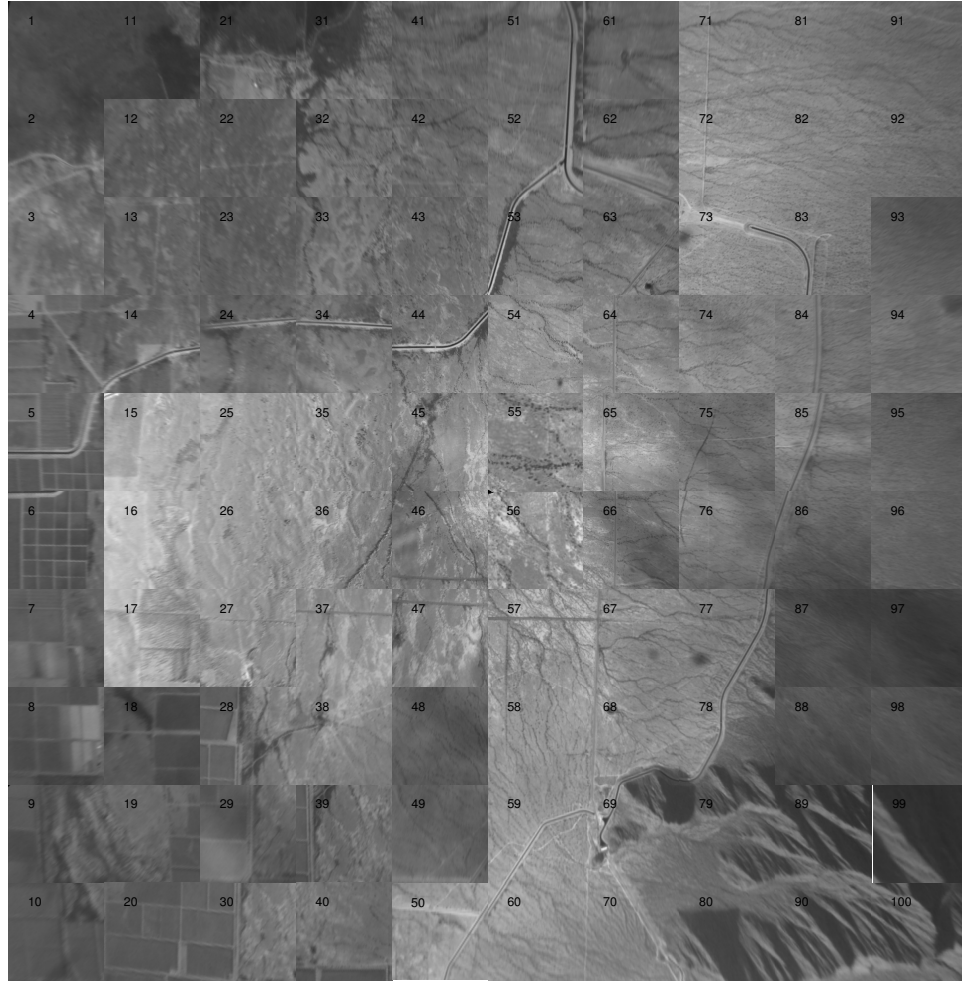
Figure 5.4: Map of similar area as shown in Figure 5.1, with tiles composed entirely of camera images projected to the ground plane (Figure 5.3).
