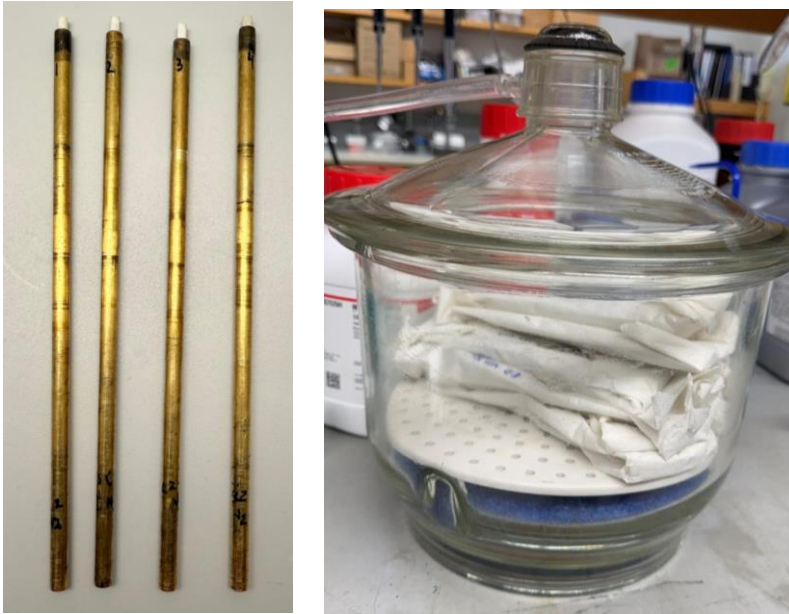
Figure 8. Metal rods glued with resin pins. Vacuum Desiccator.
