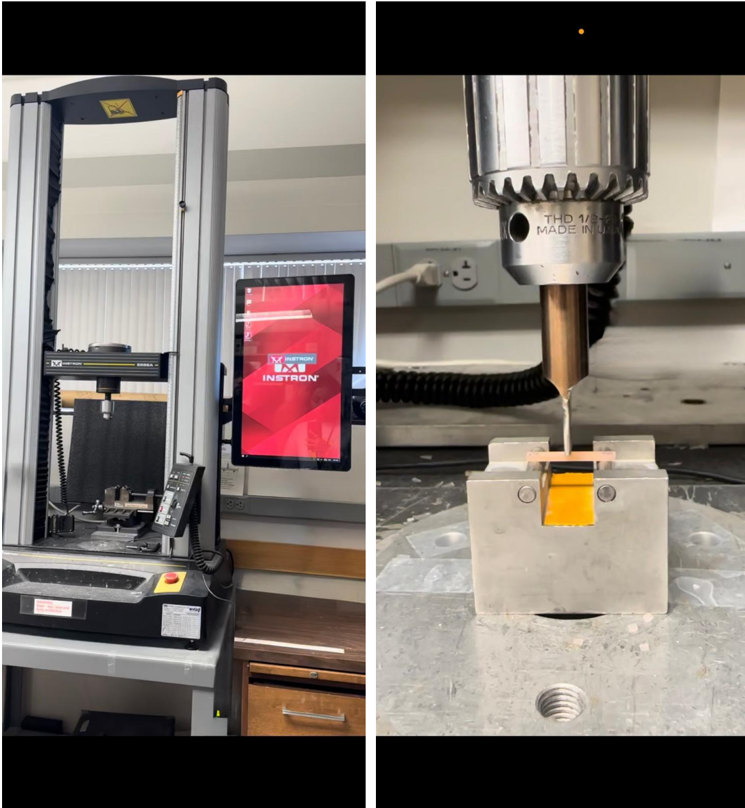
Figure 5. 5566A electromechanical Universal Tester. 20mm support jig with stainless steel rollers.
