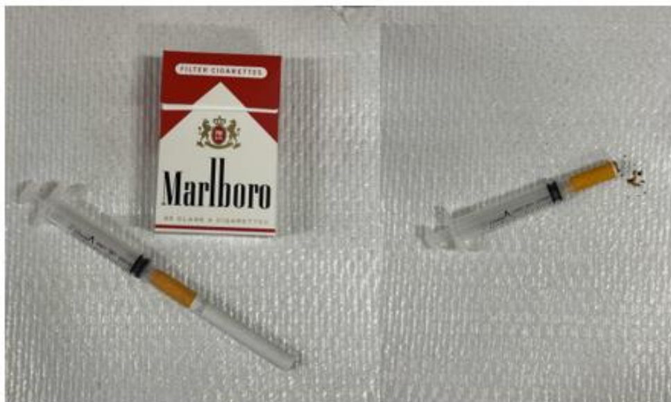
Figure 3. Image of Handheld Smoking Apparatus. (Left) A Marlboro Red cigarette, unsmoked, inserted into the handheld smoking apparatus; and (Right) the same cigarette, now consumed down to the butt, still inserted into the handheld smoking apparatus.
