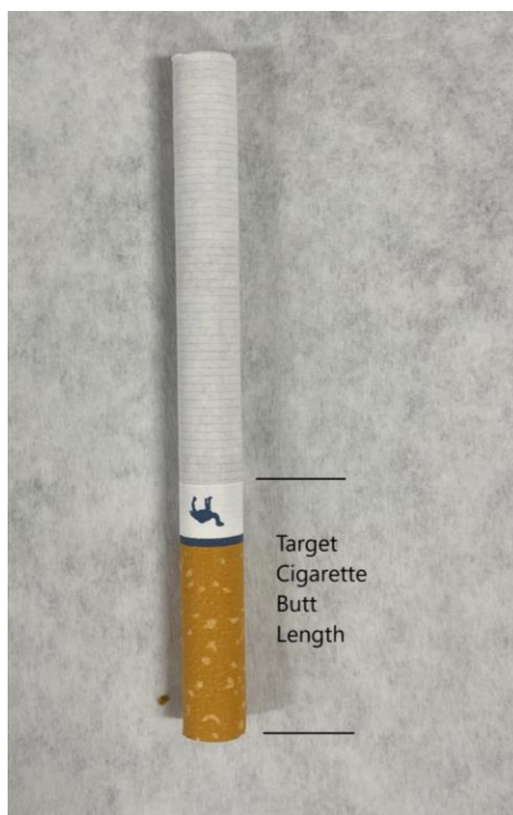
Figure 5. Image of Target Area for Smoked Cigarettes. A visual identifier of where each cigarette should be smoked to. Before smoking, each cigarette was compared to the area written on the bench paper.
