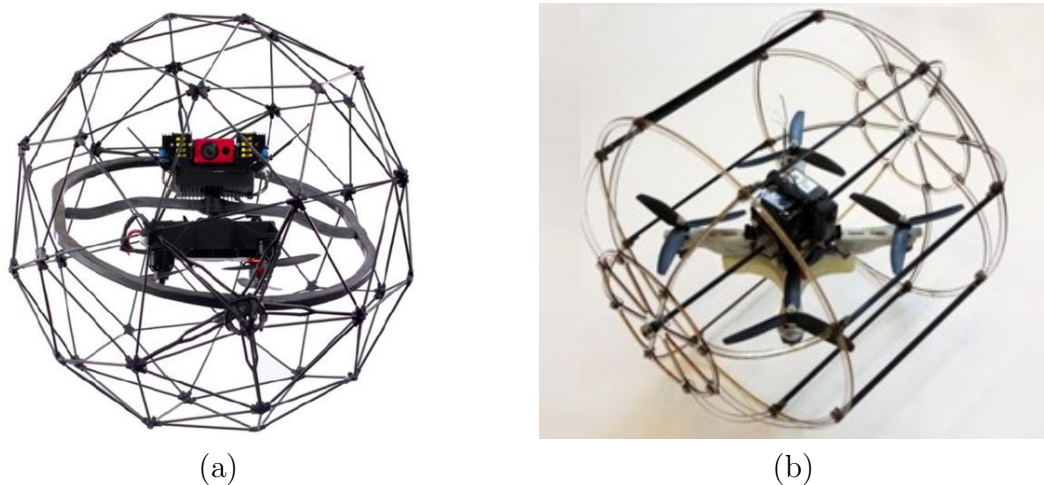
Figure 2.1: (a) Elios UAV - a collision tolerant structure (b) the HyTAQ - hybrid terrestrial and aerial quadrotor
