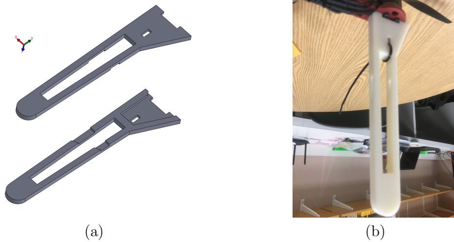
Figure 2-15: Protective frame: (a) 3D model (b) printed part
