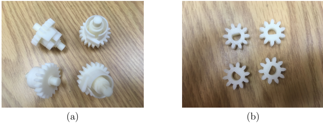
Figure 2-11: Printed gear train: (a) driving gear (b) driven gear
