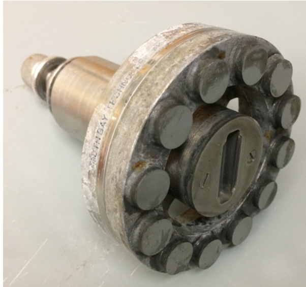
Figure A-4: Mount used for grinding the back face of the sample after titanium diffusion.
