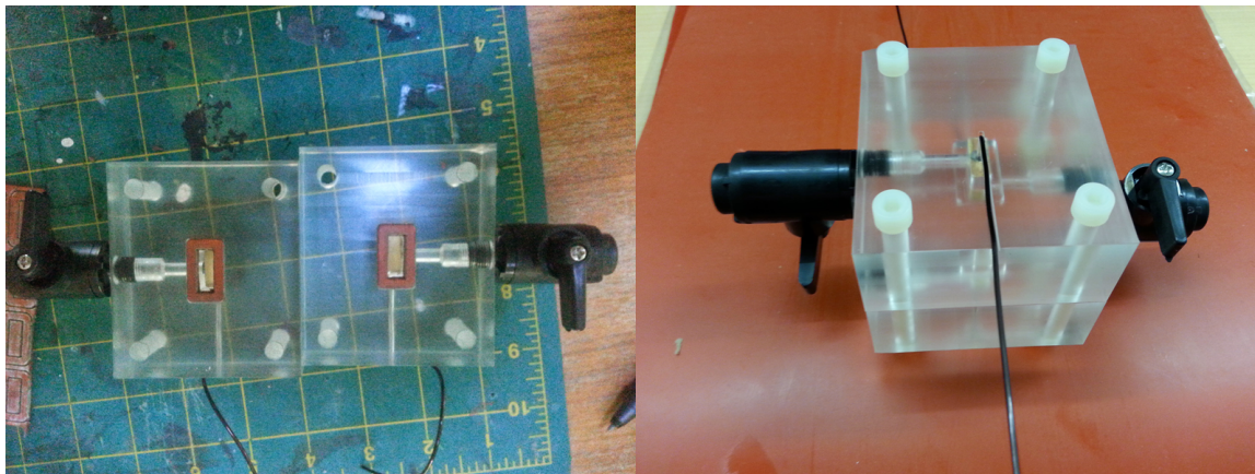
Figure A-5: Left: the halves of the poling chamber, with gaskets. Right: the assembled poling chamber.
