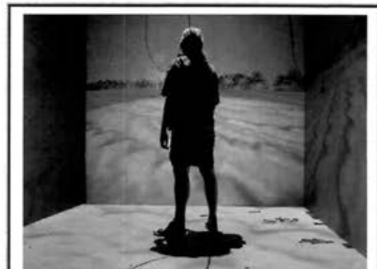
Image 2.3. Another type of virtual reality wherein images are projected on the walls. The user wears special goggles and gloves to manipulate a virtual object. (www.electronics.howstuffworks.com)
