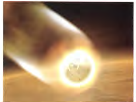
The capsule containing NASA's space rover Spirit descended through the upper regions of the Martian atmosphere at twenty times the speed of sound, cutting a largely horizontal path so that the atmosphere could absorb its speed.
