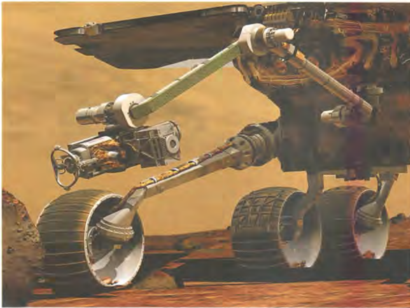
The robotic arms on both the Spirit and Opportunity Mars exploration rovers have instruments that can grind away rock layers, take microscopic images, and analyze the elemental composition of rock and soil. Illustration courtesy of NASA
