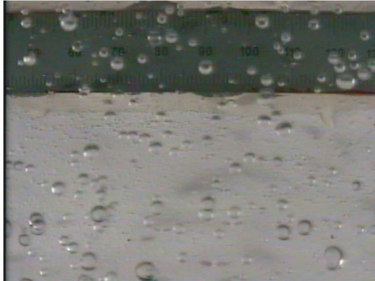
Figure 4.17: Sample frame of video captured by the underwater digital camera for a supply pressure of 9.0 psi. The machinist's scale is visible at the top, perhaps appearing as a dark band in poor reproductions of the figure.
