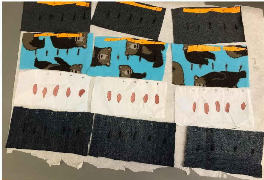
Figure 1. Preparation of stains. Five blood and saliva mixture stains on twelve fabric swatches (top to bottom): three spandex, three fleece, three cotton, cotton, and three denim.
