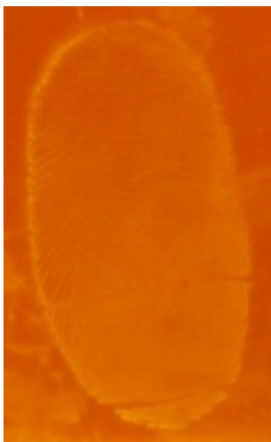
Figure 15: Lumicyano on White Tile Subsequent to Lumicyano™ Fuming Viewed with Blue Crime-lite™ with Orange Filter
