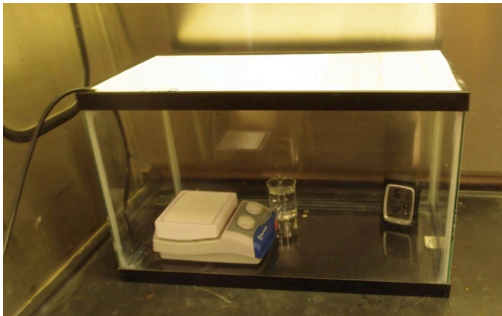
Figure 4: Enclosed Fuming Chamber
