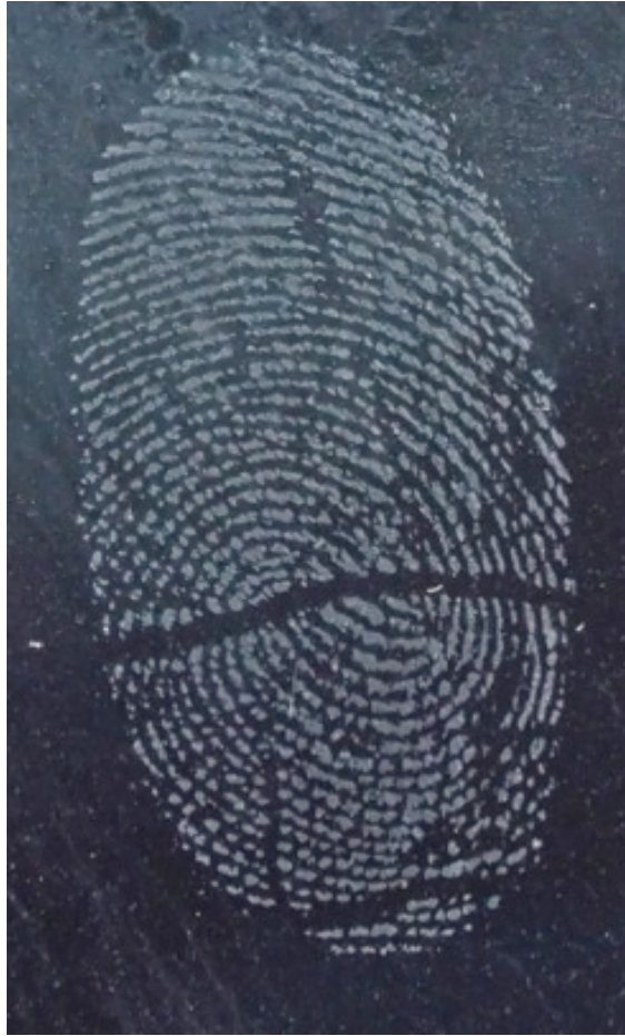
Figure 3: Cyanoacrylate Polymer Formation on Black Ceramic Tile
