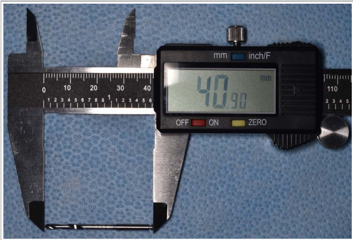
Figure 5. The length of the Nobel 2.0mm pilot drill used in BU clinic measured 40.9mm with the Boley Gauge
