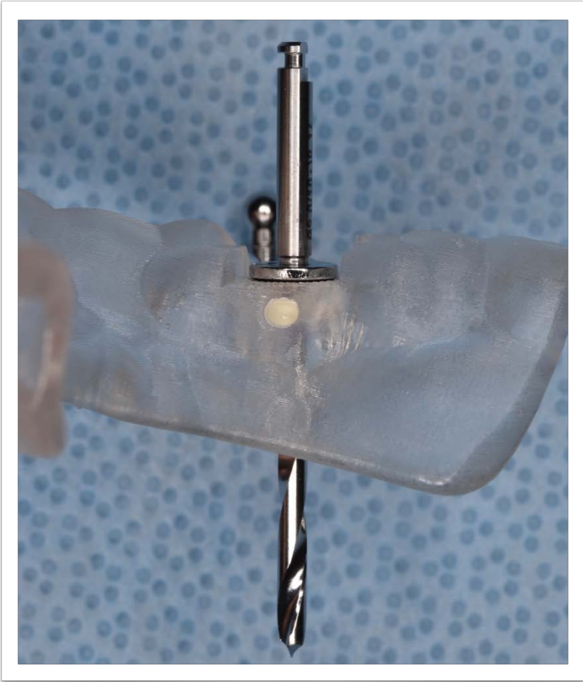
Figure 7. Nobel 2.0mm pilot drill, Nobel Surgical Guide, and Nobel guide reduction sleeve RP 2.0mm top to bottom (from lingual)
