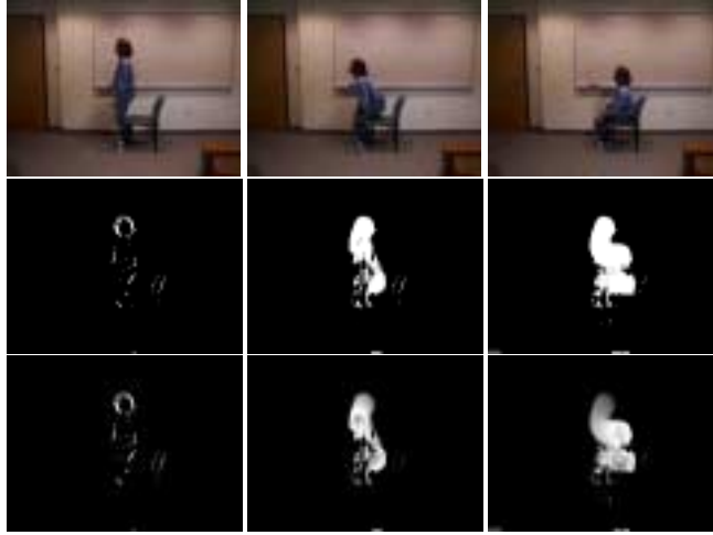
Figure 1: Sitting-on-chair action. Top row shows single frames of the action, middle and bottom row contain their respective MEI's and MHI's calculated up to the given frame. Notice that MEI's are just a thresholded version of the MHI's
