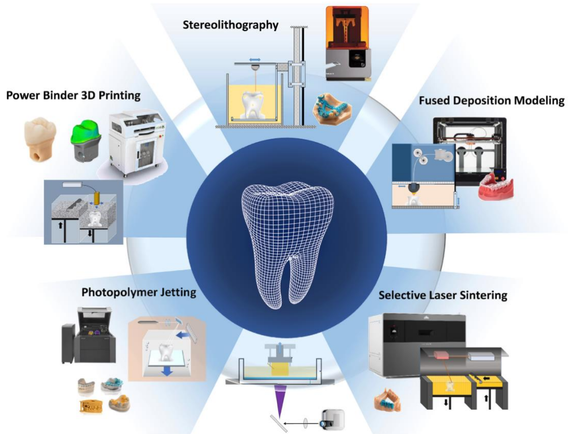
Figure 1: The Different 3D/4D Printing Techniques Used in Dental Applications. This figure projects various and current 3D printers; each adopts different methods for producing dental prosthetics, oral appliances, and artificial tooth-supporting tissues (crowns, bridges, implants, orthodontic appliances, and alveolar bone). (Figure taken from Khorsandi et al., 2020)
