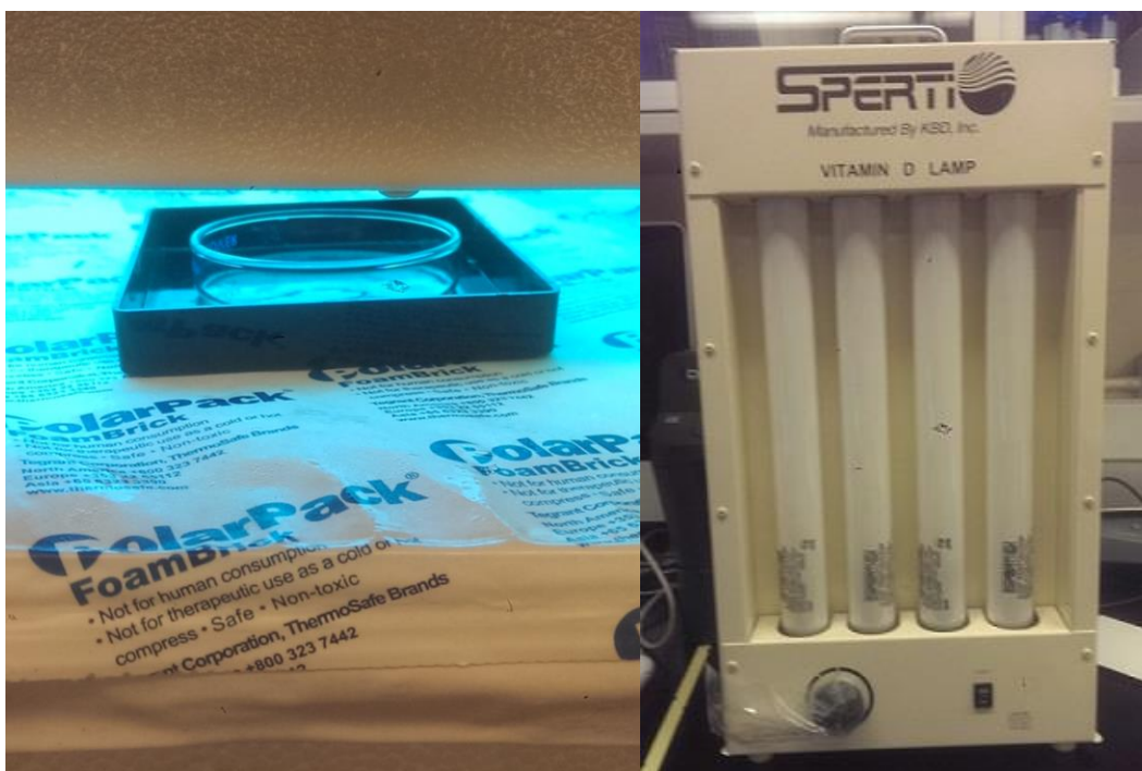
Figure 10 Synthesis of Tachysterol and Lumisterol. (Left) 7-Dehydrocholesterol was irradiated under the Sperti UV-Lamp by KBD, Inc. for 45 minutes over an ice pack to reduce conversion of previtamin D 3 to vitamin D 3 . (Right) The Sperti lamp used in preparing the stock solutions.
