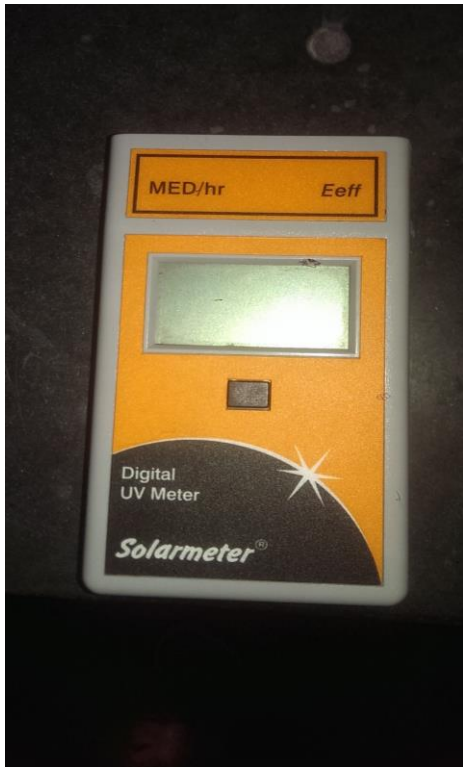
Figure 12 Solarmeter used to gauge the MED/hr during each day of the study
