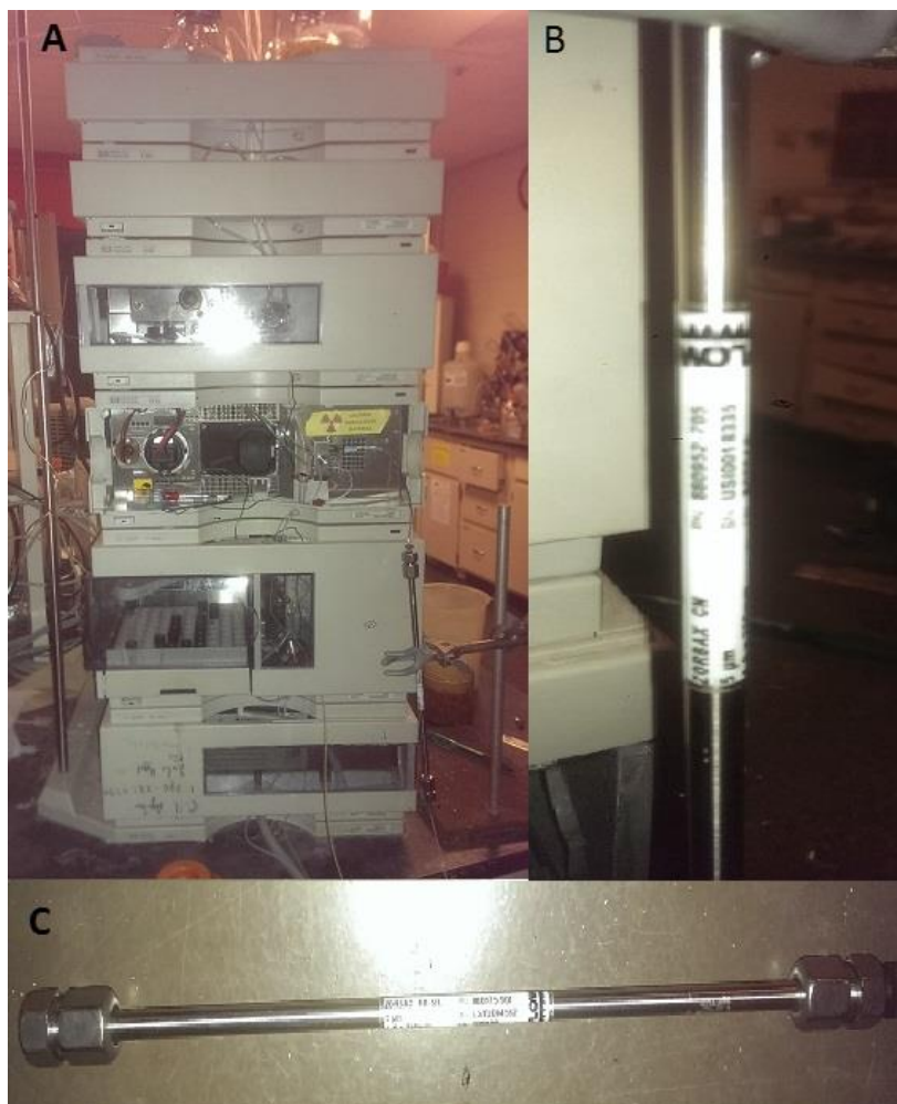
Figure 11 The HPLC setup for isolation, identification, and quantification of products within the vitamin D field: (A) the main unit consisting of the autosampler, pump, degasser, and variable wavelength detector. (B) Zorbax CN column used to separate vitamin D 3 from tachysterol 3 . (C) Zorbax RX-Sil column used to separate previtamin D 3 from lumisterol 3 .
