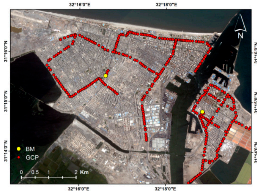
Figure 4. Two benchmarks (BM) were used as reference points for the 347 GCPs.
