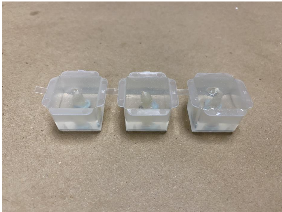
Figure 4 Embedment of the Samples in Resin Blocks
