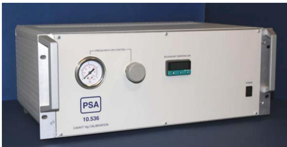
Figure 48 PSA 10.536L Hg generator
