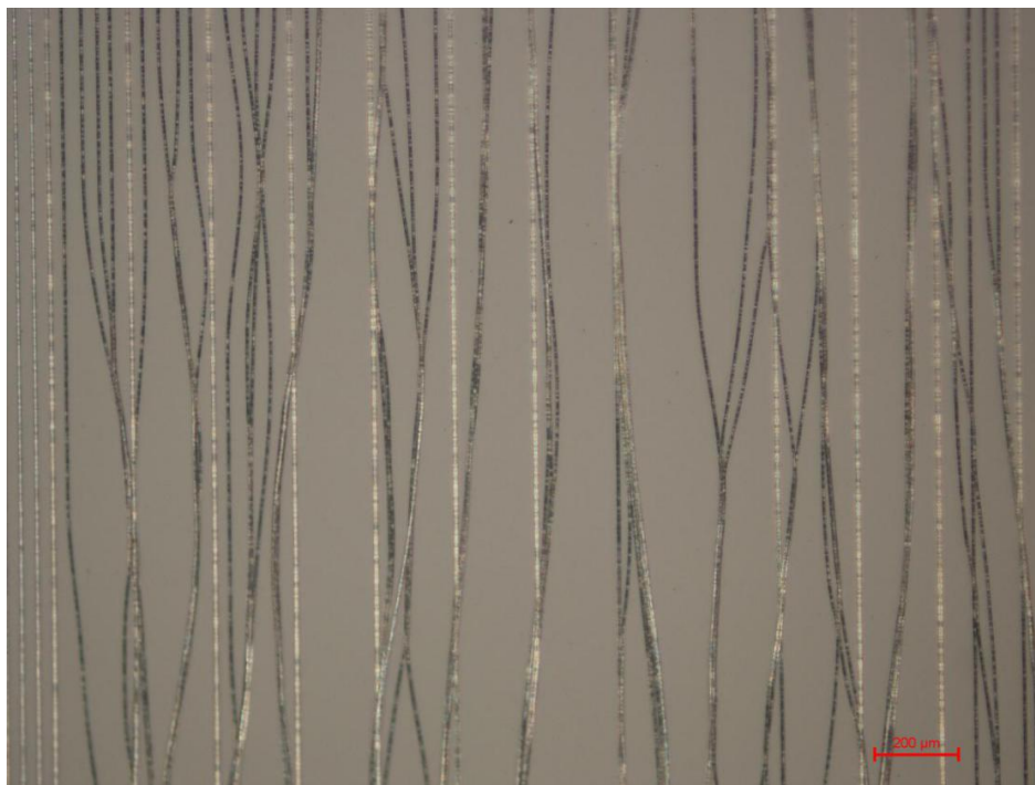
Figure 39 Microscope figure of IDT patterns on ST-cut quartz wafer with 3 s exposure time and 1 min hard bake
