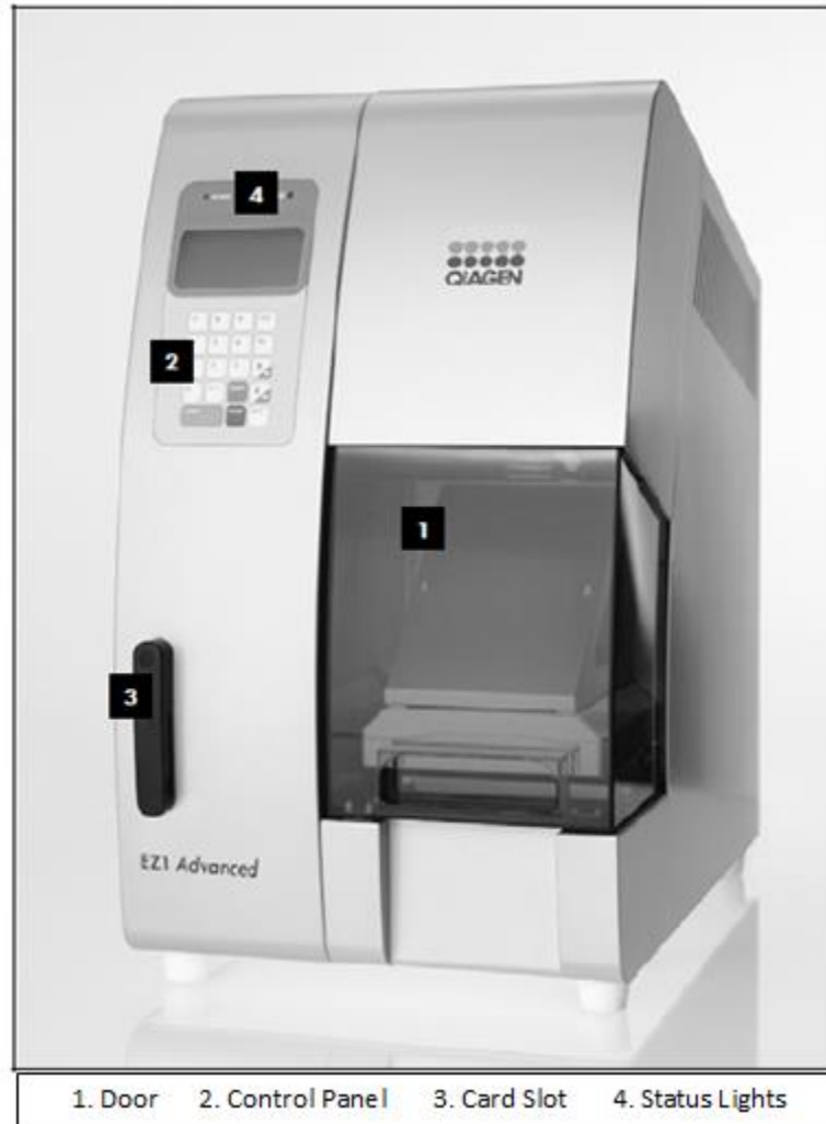
Figure 2: Overview of the QIAGEN® EZ1® Advanced Bio-Robot (QIAGEN®, Hilden, Germany) Photo obtained from the Qiagen EZ1® manual and depicts the door, control panel, card slot and the status LEDs (16).
