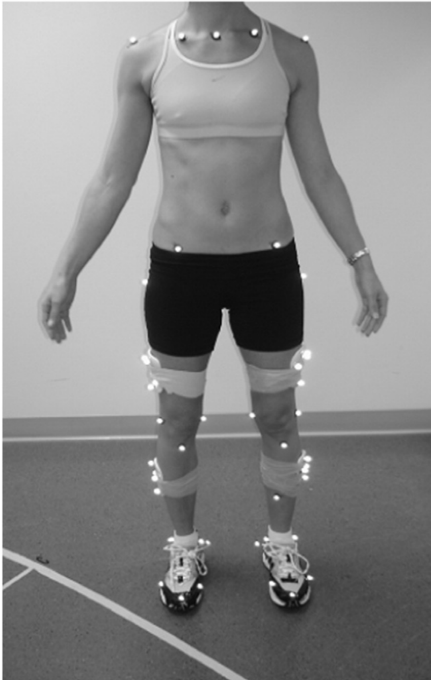
Figure 2. The marker set-up used to track motions at the pelvis, femoral region, and tibial region. Taken from (Brown et al., 2016)
