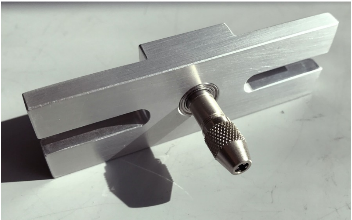
Figure 5-2: Commutator built with low-friction, precision ball bearings allows fiber to rotate. A passive commutator constructed with precision ball bearings holds the ferrule and polished imaging surface below a microscope objective. As the animal moves about the enclosure, the fiber can freely rotate, while remaining level in the focal plane of the microscope.
