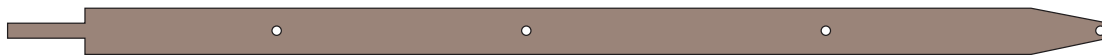
Figure 5-1: A diagram of a prepared polyimide strip to reinforce a chronic fiber bundle implant. A strip of polyimide is used to absorb physical stresses, protecting the bundle of fibers. The fiber bundle is threaded through the small holes and the bottom hole (right) is used to anchor the polyimide strip to the skull.
