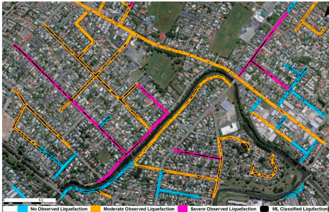
Figure 14. Liquefaction severity observation on the roads after the event by reconnaissance team along with the classified liquefaction using ML classifier on the satellite imagery.
