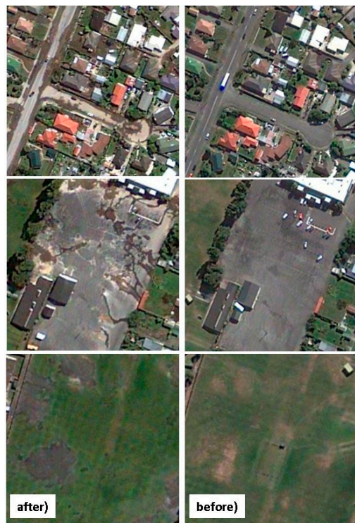
Figure 4. Satellite imagery before (14 February, 2011) and after (23 February, 2011) the Christchurch earthquake. Liquefied materials on the ground can be seen. Images from Google Earth. Note that these imageries are selected very close to the earthquake event date for only sake of showing the meaning of earthquake-induced liquefaction. These imageries are not use in this study for classification as they do not have any spectral information associated with them.
