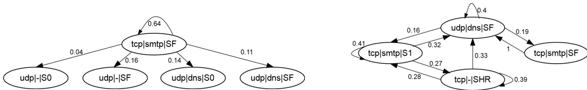
Figure 11: Markov Chain for Sality (right) and Geodo (left) spam behavior (only state transition probabilities, where p > 0.1 ).
