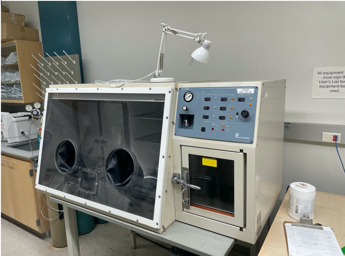
Figure 1. Anaerobic Chamber used to culture multi-bacterial mixture that was introduced to exposed mouse pulp chambers for inducing endodontic infection.
