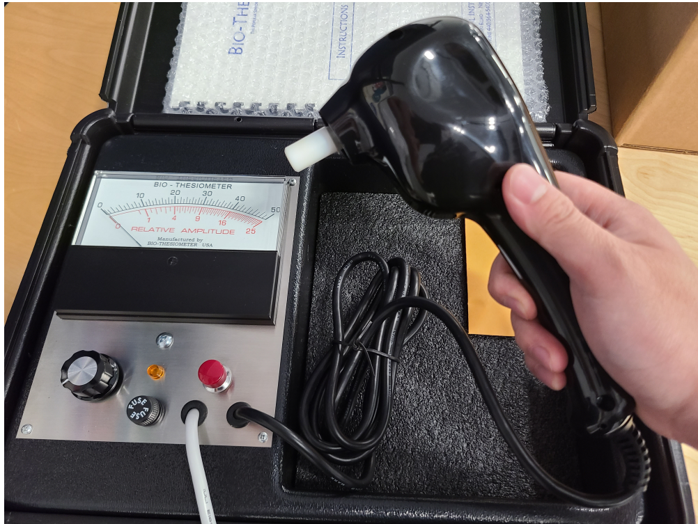
Figure 3. An image of a biothesiometer for use in the VPT test. The probe tip vibrates at a constant rate while the intensity of the vibration is adjusted with changing the voltage.
