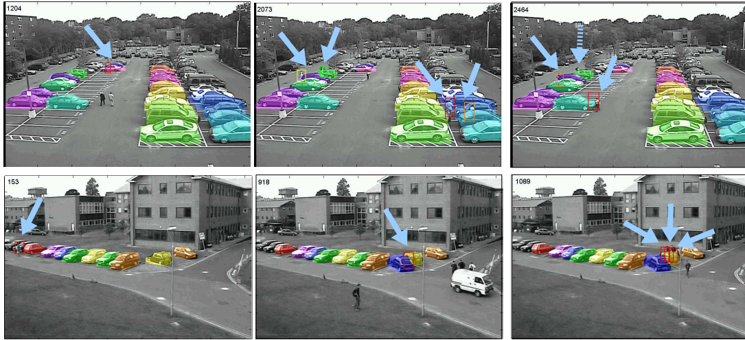
Figure 6-2: Example frames from our tracking algorithm applied to test video (a), top row, and to test video (e), the PETS 2001 sequence, bottom row. Rectangles indicate observation regions corresponding to the ground-plane zones selected by the tracker; the color of these rectangles in each frame is chosen for visual contrast. A missed pedestrian is marked with a dashed arrow; correct detections are marked with solid arrows.
