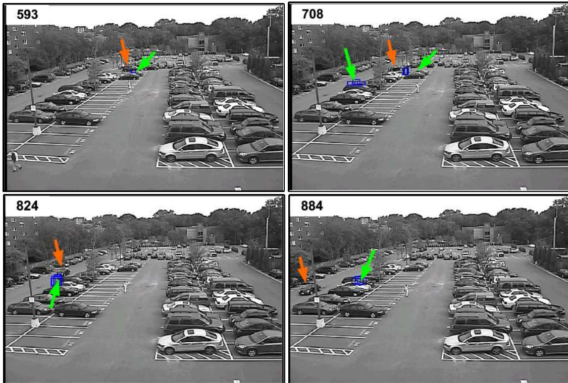
Figure 5-5: Tracking results for the “far-field” test video sequence from the COP2007 dataset are visualized as samples of p(\mathbf{Y}_t|Z_{1:t}) in the Markov chain. Green (light) arrows point to the image-truth locations of the two pedestrians in the scene; orange (dark) arrows point to the moving vehicle.
