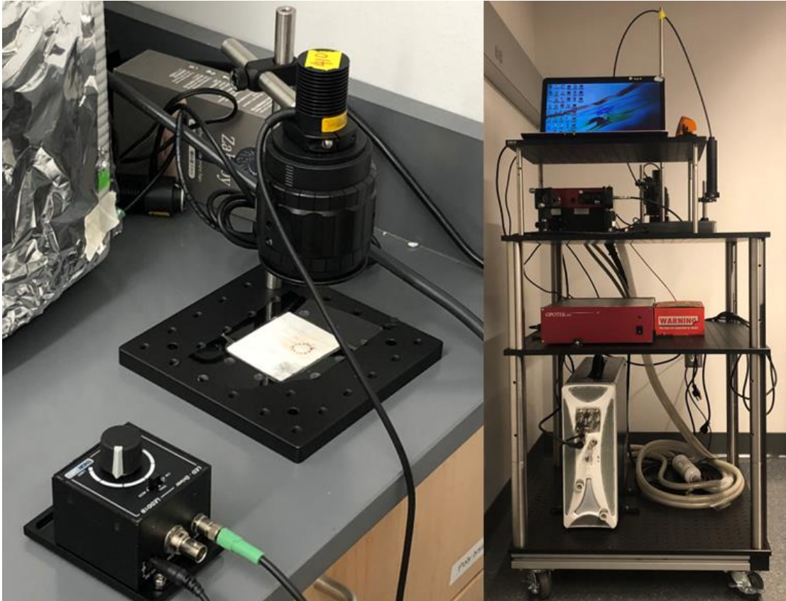
Blue light application devices used in bacterial and fungal studies. Left) 405 nm LED system used to deliver continuous wave light to pathogens within in vitro and in vivo environments. Right) Tunable nanosecond pulsed laser device allowed for delivery of blue light between 410 and 480 nm.
