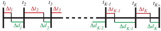
Figure 2-1: Time sequence of a single agent on a given trajectory. The t_j are the time points where the agent begins to move to the next target in the sequence. Each move takes \Delta t_j units of time followed by a dwell period of \Delta d_j units of time during which information is collected from the target.
