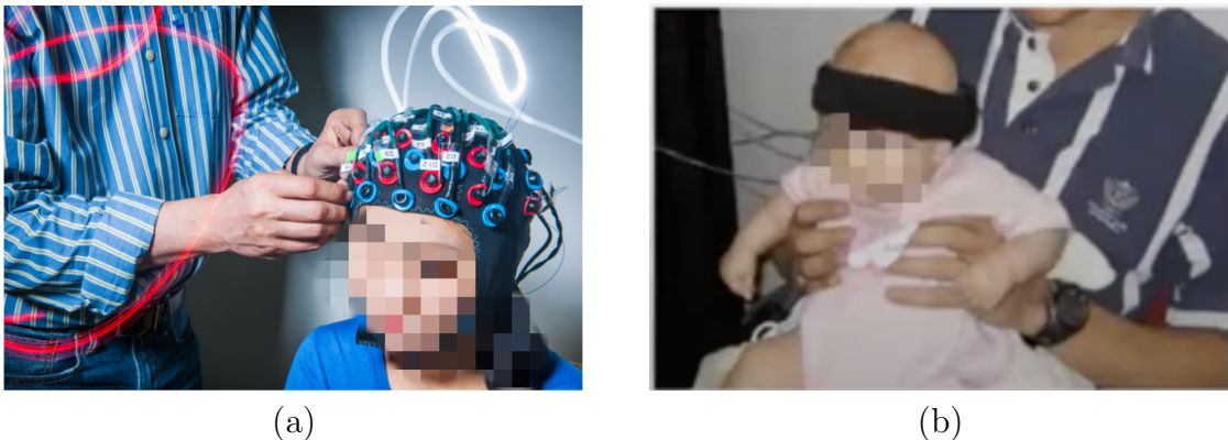
Figure 1-1: The current state-of-the art fNIRS systems (a) The cutting edge multi-channel fNIRS measurement system to measure adults; and (b) fNIRS systems that are commonly used for infants.
