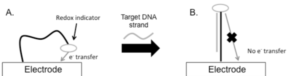
Figure 11. A schematic showing the effect of the hybridization of the target strand to the recognition layer. A) Without the target strand the redox indicator (methylene blue) will interact with the surface of the electrode causing electrons to transfer between the two producing a current. B) After the target is hybridized there is no electron transfer between the redox indicator and the surface thus causing less current to be produced and a decrease in the signal observed [57].
