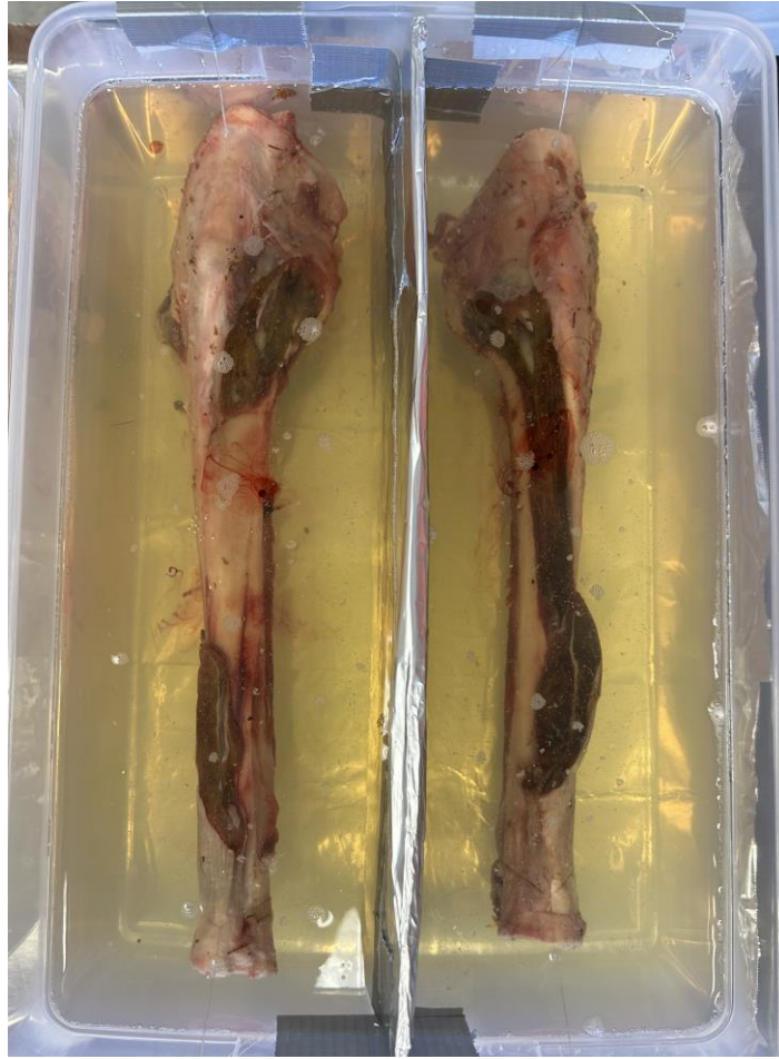
Figure 1. Two deer tibiae are embedded in 10 cm of ballistic gelatin. The anterior aspects are approximately 5 cm below the surface. There is an aluminum divider between the two tibiae, so they can each be impacted separately.
