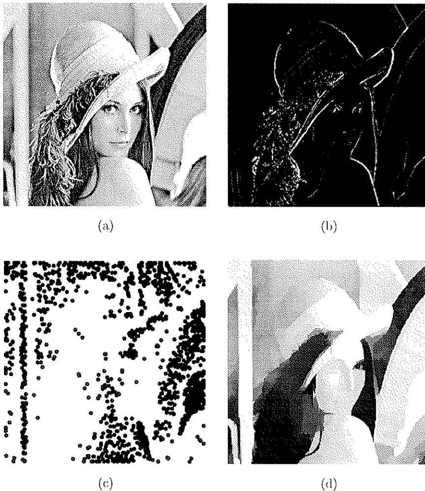
Figure 3.4: Anisotropic interpolation of an image based on very sparse sampling. (a) Original Lena image. (b): Magnitude of image gradient. (c): Samples taken from lowest magnitude points. (d): Anisotropically interpolated image.
