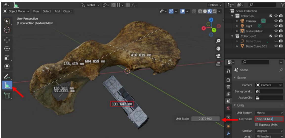
Figure 3. Use of the measure tool to adjust the global unit scale with Individual BU35-L.
