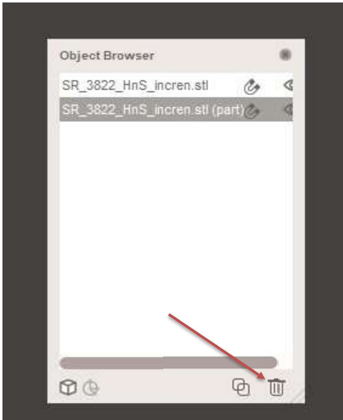
Figure 7. Separate object browser in Meshmixer. Once the separation occurs, meshmixer views the highlighted region and the non-highlighted region as two different entities. The object browser will appear on the right lower corner of the screen to indicate this. From here, users can click on the part they do not want to keep and delete it via the delete button (arrow).
