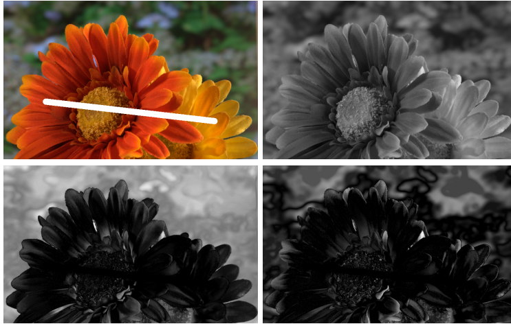
Fig. 3. Top left: “Flower” image (from Rhemann et al. [3]) with seedpoints overlaid in white. Top right: Gray-scale image. Bottom left: BMD distance transform of the color image, after transformation to the CIEL*a*b* color space. Bottom right: BMD distance transform of the gray-scale image. The values of both distance transforms have been scaled for display purposes. Compared to the single-channel distance transform, the multi-channel BMD distance transform better captures the contrast between the flower and the background.
