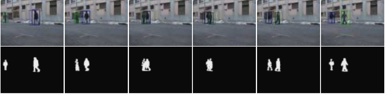
Figure 4: Tracking example: input sequence, and blob segmentation results.
