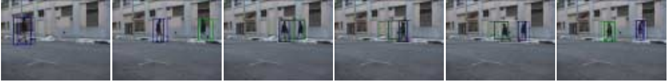
Figure 8: Tracking results, non-linear trajectories. Bodies are tracked, but prediction is less accurate because of sudden change in direction during occlusion.
