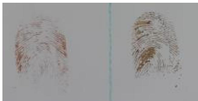
Figure 17. Discoloration of bloody prints after application of 5-SSA fixative. Left: Before fixing. Right: After fixing with 5SSA.
