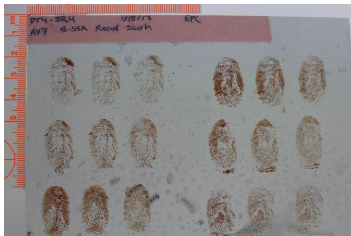
Figure 11. Image of the metal piece with bloody prints applied over dried road slush contaminant. All bloody fingerprints applied over contamination.
