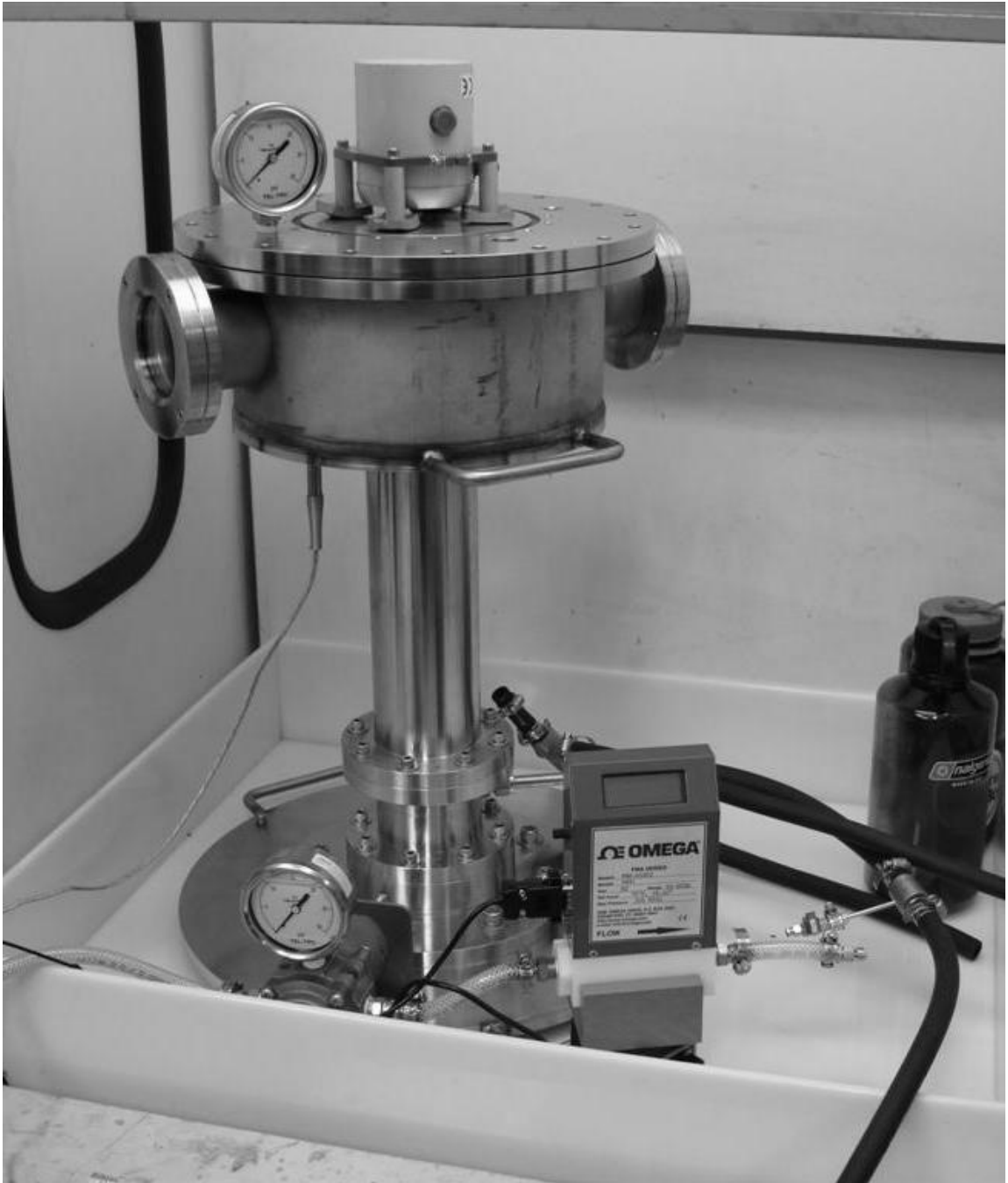
Figure 3.6: The acoustic resonator assembly. In this particular photograph the shaker cover is not attached, and the reservoir outlet tubing is disconnected.
